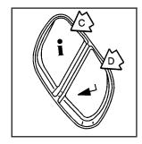
A **TN** (**Trip Information**): Press this button to display the odometer, trip odometers, tire pressure for vehicles equipped with a tire pressure monitor, timer and engine hours.
